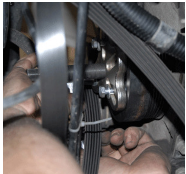
ONLY IF YOU HAVE A WINDSOR ENGINE, use a balancer removal tool to remove the factory harmonic balancer and set aside. It will not be reused. Those with the Romeo engines do not need to remove the balancer.
