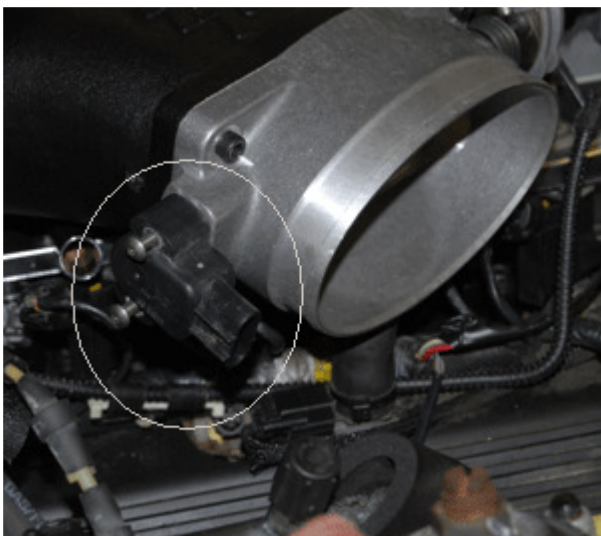
Attach the throttle cable and cruise control cables to the throttle body using the provided adapters.
