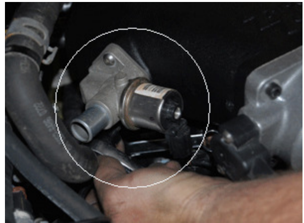
Install the Throttle Position Sensor and the Idle Air Control Valve to the throttle body and inlet plenum and connect electrical harnesses
