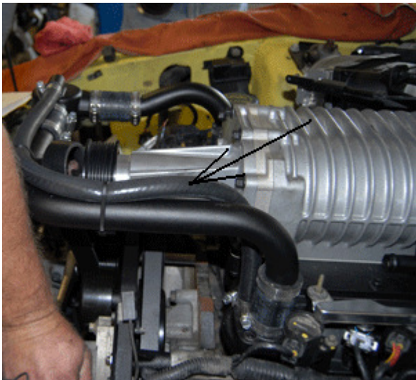
Install the coolant bypass hose (see arrow) from top of Tstat housing to the left of the driver's side coolant tube.
