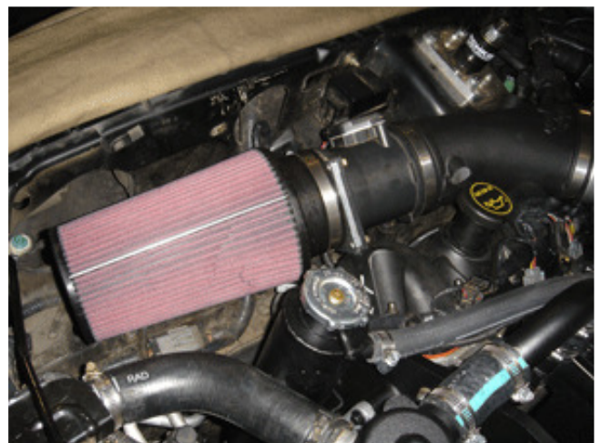
Attach filter to the MAFS and install the optional air filter guard (Air Divider), if purchased. Note that the MAFS will need to be rotated slightly so it fits as low as possible in the engine bay without interfering with the cam covers. See the picture above as a reference.
