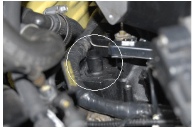
Attach the remaining coolant line going to the heater core on the fire wall to the fitting on the back of the passenger side manifold. Secure with a clamp. The stock hose is reused.
