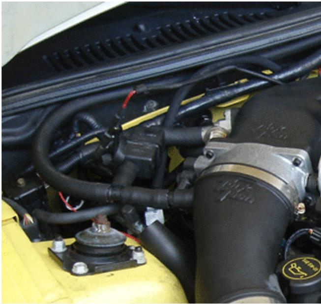
Idle air control to intake tube to passenger side cam cover vacuum circuit. You will insert a male/male fitting into the
