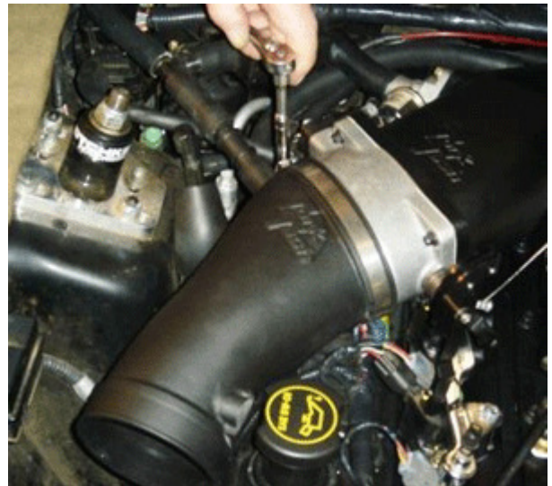
Install the intake tube to the throttle body and the MAFS/adaptor to the new intake tube. The vacuum fitting on the tube is very close to the TPS but the tube can be rotated slightly so it does not interfere.
