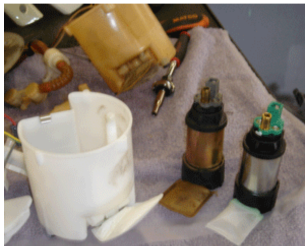
New pump on right with new filter is inserted into old basket.
