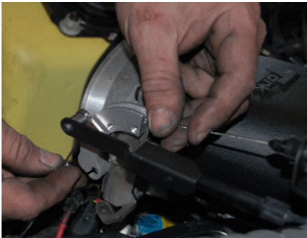
Attach the throttle cable and cruise control cables to the throttle body using the provided adapters.
