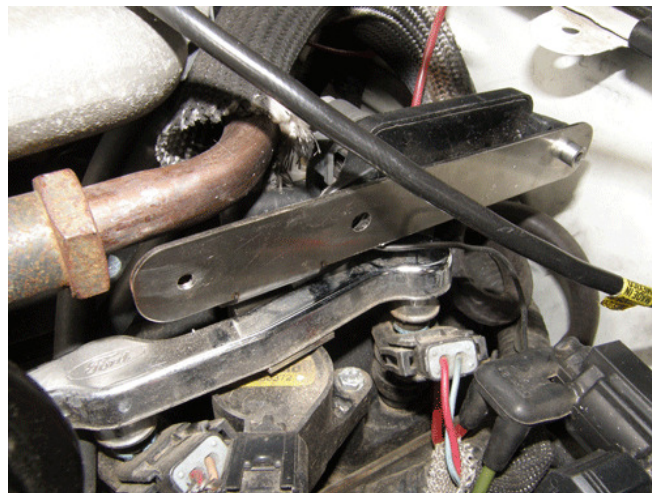
Bracket shown attached to the fuel rail bolt/stud. Note the center bolt will hold both the transducer and the solenoid so install it last!
