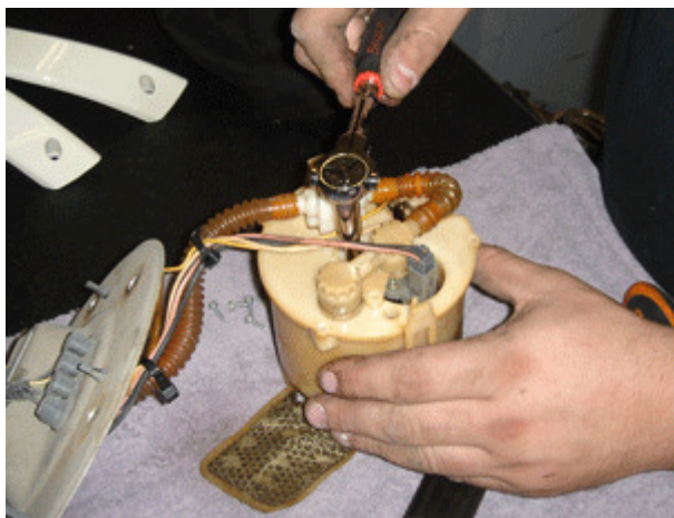
Remove the screws that hold the top to the lower basket on the original fuel pump.
