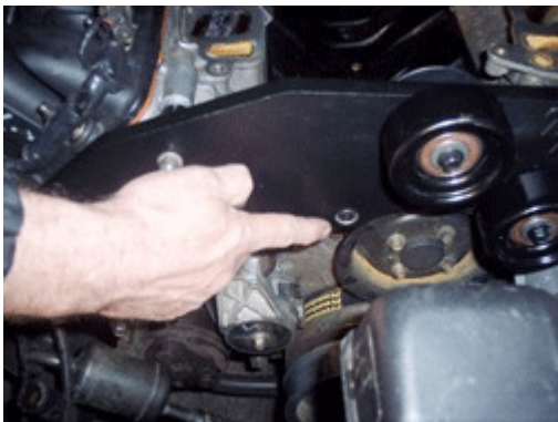
Install the cross brace using the two long bolts and thread them into the upper front cover tapped holes and fasten to approx. 25 ft-lb. We recommend installing a NEW accessory belt and the belt needs to be positioned now for proper routing and installations shortly. There is a third attaching point for the cross brace in the middle. Attach the long center Allen head bolt into the recessed hole and the stiffening sleeve that goes back to the block, but first place your new belt into position so the bolt/sleeve is in the middle of the belt. The Allen bolt and sleeve is individually
